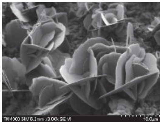
Accelerating voltage: 5 kV Image signal: SE Magnification: 3,000x Sample: Copper crystal (Copper sulfide)
