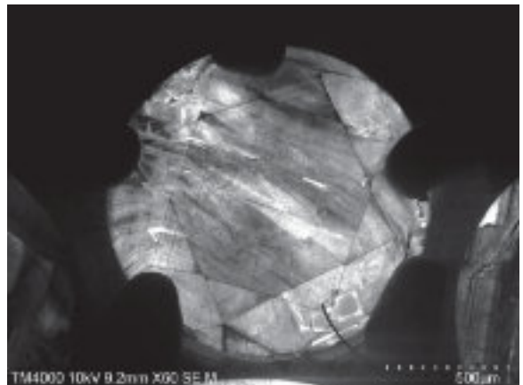
Accelerating voltage: 10 kV Sample: Diamond Ring Image signal: UVD-CL Magnification: 60x
