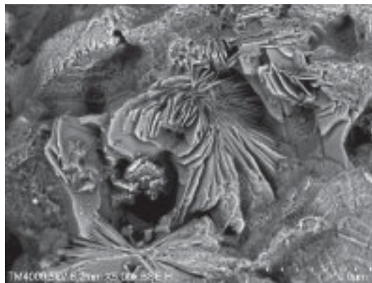
Accelerating voltage: 5 kV Image signal: BSE Magnification: 5,000x Sample: Cement Secondary electron images and MIX images can only be observed in TM4000Plus II *Option
