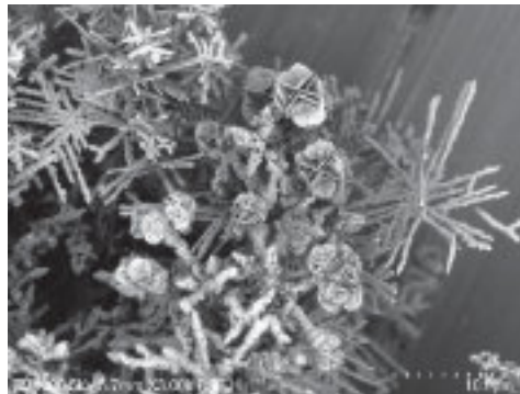
Accelerating voltage: 5 kV Sample: Copper crystal Image signal: BSE Maghification: 3,000x
