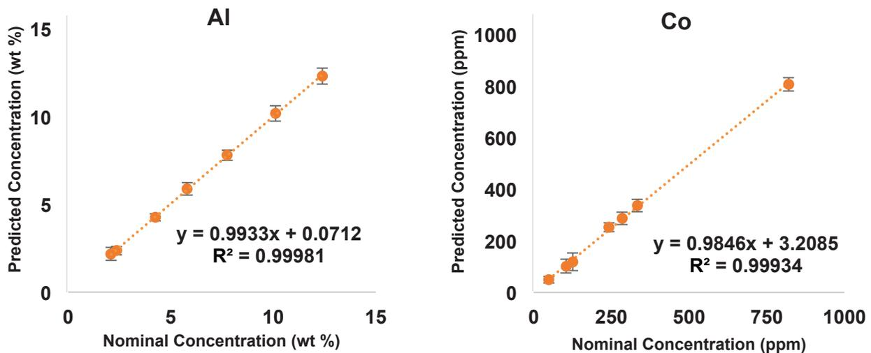
Figure 3. Multivariate calibration curves for Al (2.09 – 12.4 wt. %) and Co (49 – 820 ppm).
