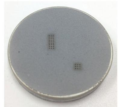
Pressed Pellet: Post sampling; 9x3 and 3x3 laser-sampling grid.
