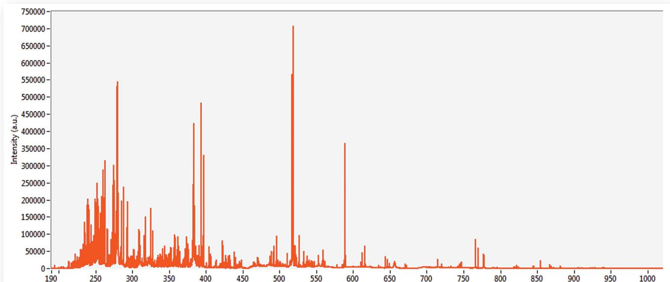
Figure 1. Typical LIBS spectrum of AMIS 171 acquired with the J200 LIBS instrument.
