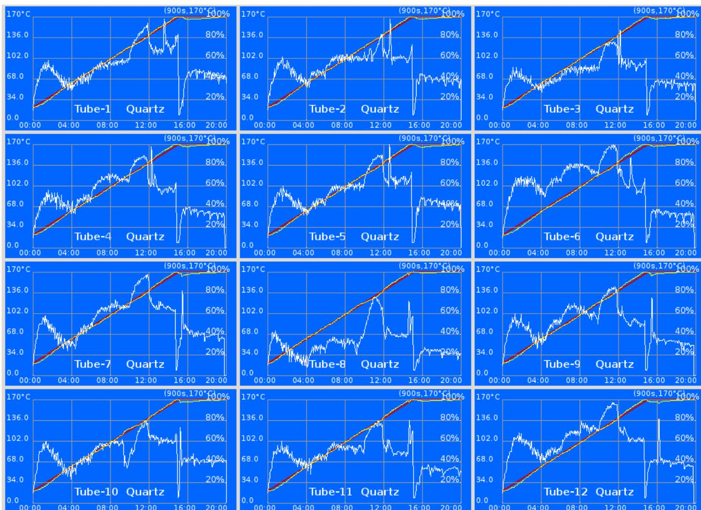
Method: USEPA 3015A; Vessel Type: Quartz; M/V: 0.5 g of Soil, 5 ml HNO<sub>3</sub>, 45 ml Water.
